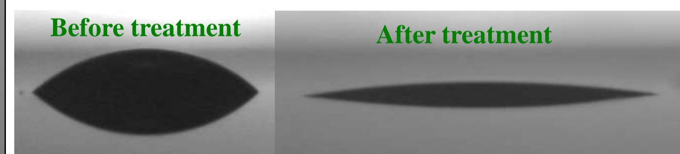
Contact angle of a water droplet at the surface of glass before and after microplasma treatment.
